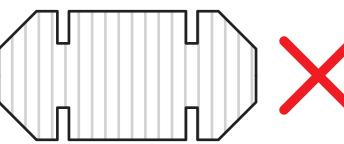
Corrugations should run perpendicular to the slots (the long way through the planks) for greatest durability.
